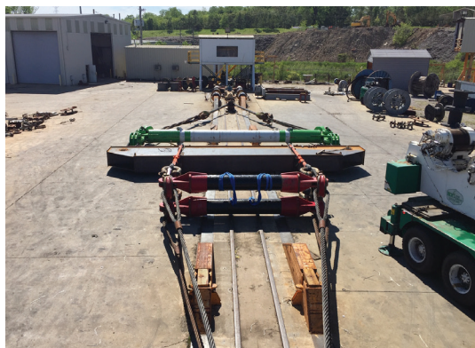
550 ton turbine lifter load test
