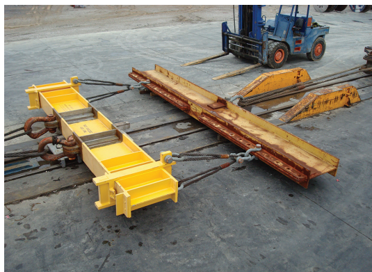
235 ton load test of a 20 ft. (yellow) turbine-lifting spreader beam
