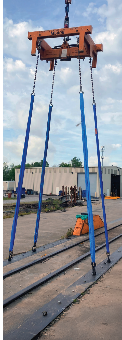
15 ton 4-point lifter vertical test
