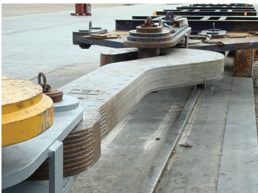
195 ton load test of a ladle hook
